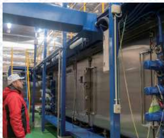
Right: The sake brewery that has introduced a machine to make koji is a rare one. This has greatly reduced the burden of koji making, which had previously required a sleepless shift. Left: Rokkasen makes a lot of Junmai Ginjo-shu using sake rice produced in the prefecture.
